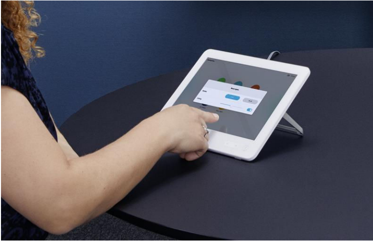
Figure 2. User interface displaying in-room control information
