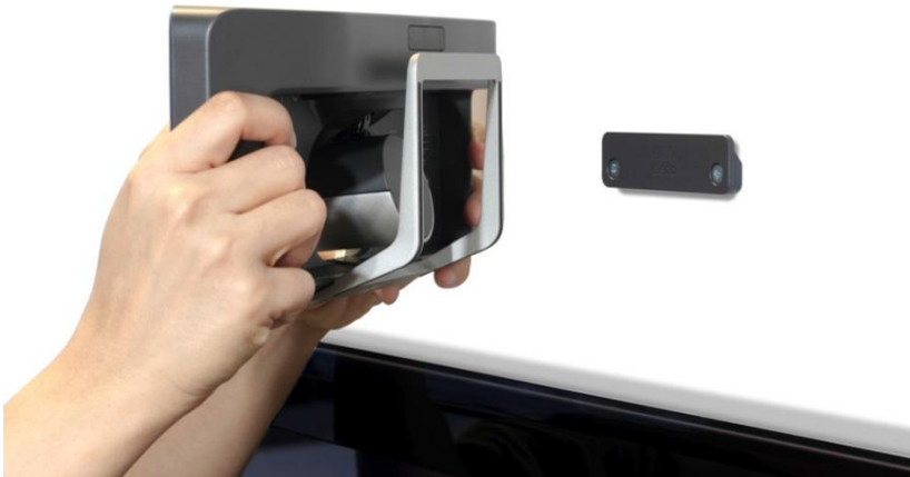
Figure 3. Cisco TelePresence SX10 Wall-Mount Solution
