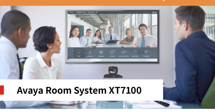
The Avaya Room System XT7100 is the flagship offering in the XT series of video conferencing room systems. The XT7100 incorporates H.265 High Efficiency Video Coding (HEVC), one of the industries most advanced video compression technologies. H.265 HEVC doubles the video compression efficiency of H.264 High Profile, enabling full HD 1080p 60fps video with half the bandwidth required<sup>1</sup>, delivering an exceptional experience with a total lower cost of ownership.
